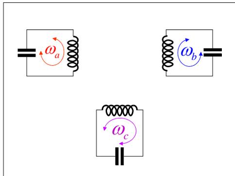
$$\frac{H_{rev}^{lin}}{\hbar} = \omega_a a^\dagger a + \omega_b b^\dagger b + \omega_c c^\dagger c$$
